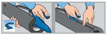
The use of the cutter is illustrated in these two diagrams. Let the blade run along the tube without the tool's surfaces touching it to get a neat, clean cut.
