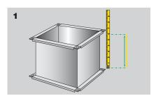
There are considerable advantages in using K-FLEX ST ROLL SHEET for ducting, which has the same height as the sheeting.
