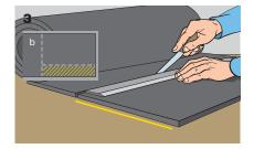
Cut the corresponding portion out of the roll. There is an obvious saving in material by cutting the sheeting along its height (a) rather than along the length of the 1000 mm sheeting (b).
