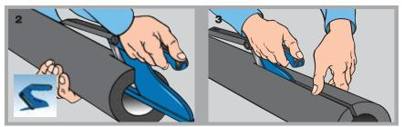
The use of the cutter is illustrated in these two diagrams. Let the blade run along the tube without the tool's surfaces touching it to get a neat, clean cut.
