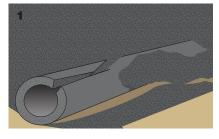
Use only the sharpest knife for cutting - this makes the subsequent glueing far easier.
