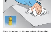
Use thinner to thoroughly clean the surface to be insulated. Insulation is not recommended where there is incrustation or other flaws which could prevent the sheeting from
